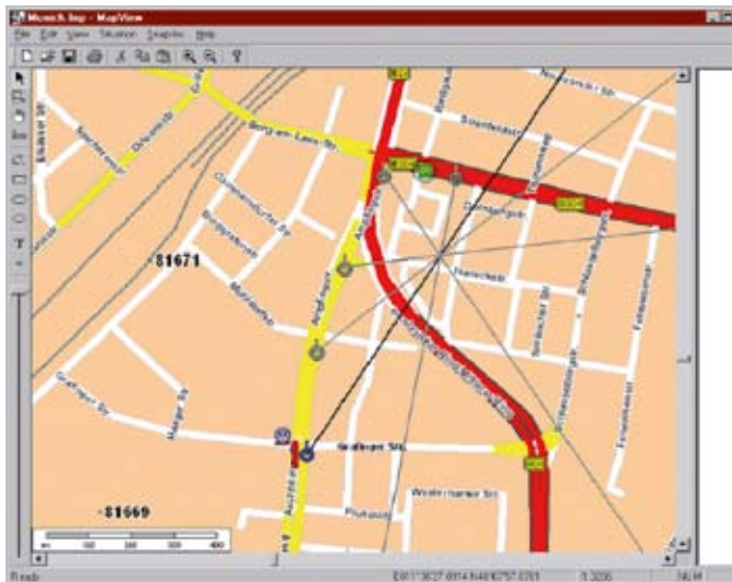
Finding the position of a TETRA terminal with running fix and display on R&S®MapView.
